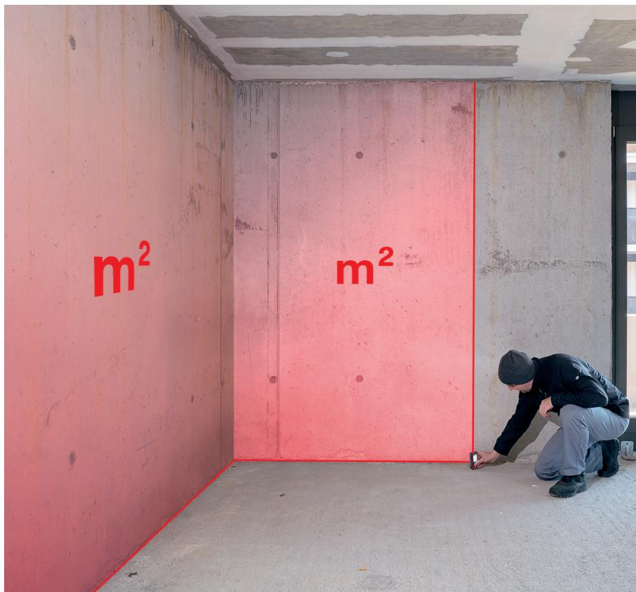
The painter function automatically calculates the total wall area of a room by adding the wall lengths and then multiplying them by the room height.
