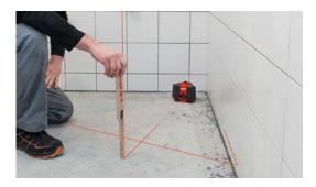
The device can also be used to quickly and easily check that floors are level thanks to its horizontal laser line, which is beamed just above the ground. The floor's properties can then be defined by using a folding rule.
