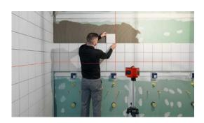
The FLOX has a 1/4" and 5/8" thread, which can be used to attach it easily on a tripod. This way, the levelled wall cross can also be used when fixing tiles to walls.
