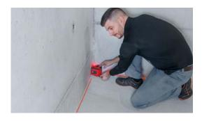
By directing the laser's floor lines close to a wall, users can easily check that the wall is perpendicular.
